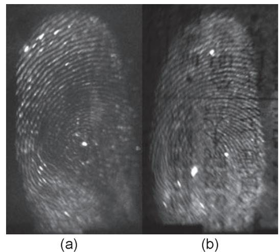
FIG. 11—Fluorescence images of fingerprints on a newspaper. (a) For color photograph page (280-nm excitation). (b) For black character page (230-nm excitation).
